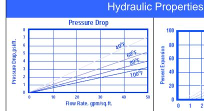
**Pressure Drop:** The graph above shows the expected pressure loss per foot of bed depth as a function of flow rate at various temperatures.
